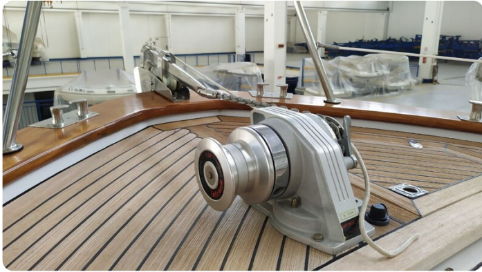
Apreamare 9 Open - Windlass Detail
